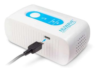
**IMPORTANT NOTE:** If after you plug the unit in and you see the green light turn on momentarily and then turn off, the unit is FULLY charged and you do not have to charge the unit. The custom battery management software will at this point, not allow the unit to take any additional charge. Your unit is ready to use.
